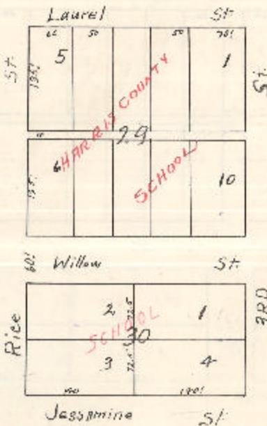
In the above plan the black lines represent the original block and lot lines and the numbers designated by the original plan. The RED LINES and RED NUMBERS indicate where said boundaries do not conform to the original lot lines. Red numbers where no part of land owned in the above block is subdivided in lots and where no other land is owned in lots and where no tract numbers are given.
